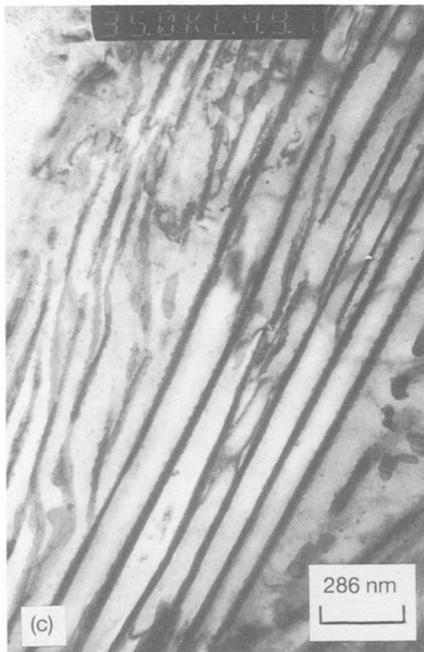
Figure 4 Lamellar pearlitic constituent for the three steels at different forging temperatures. (a) Steel 1, T_2 = 1398 K; (b) Steel 1, T_2 = 1323 K; (c) Steel 2, T_2 = 1323 K; (d) Steel 3, T_2 = 1323 K.
